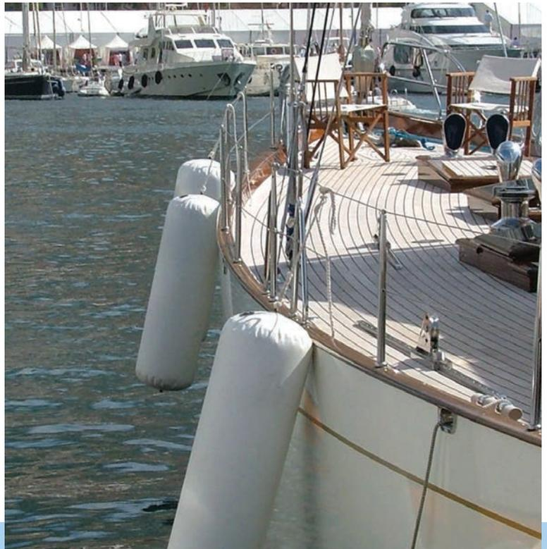
**The Magnus inflatable fenders are made of reinforced PVC material.**
